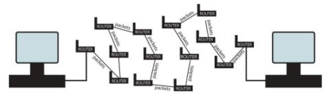
Packets travel from source to destination. Along the way, they move through different routers. They do not move together.
